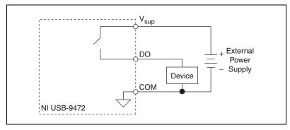
Figure 8. Connecting a Device to the NI USB-9472
